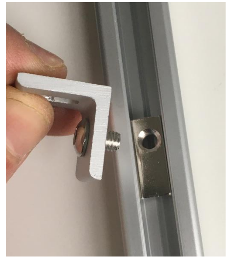
Figure 3. Attach brackets (C) using round head bolts (E).
